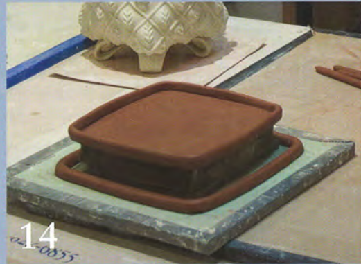
14 Place the foam inside the middle of the coil and place the top slab on top of the foam.
