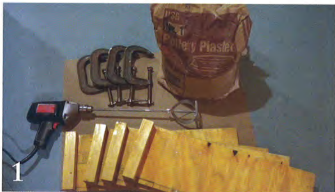
1 Build a form for your plaster mold using cottles and clamps.
