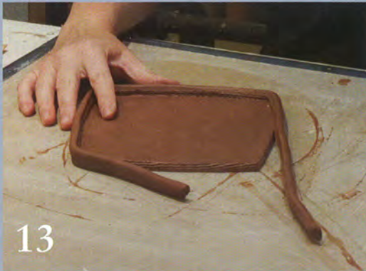
13 Score and slip the beveled coil to the edge of the slab.
