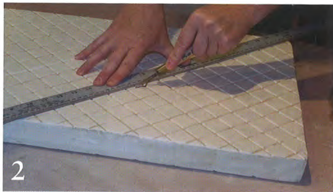
2 Create the texture grid using a loop tool and a straight edge.
