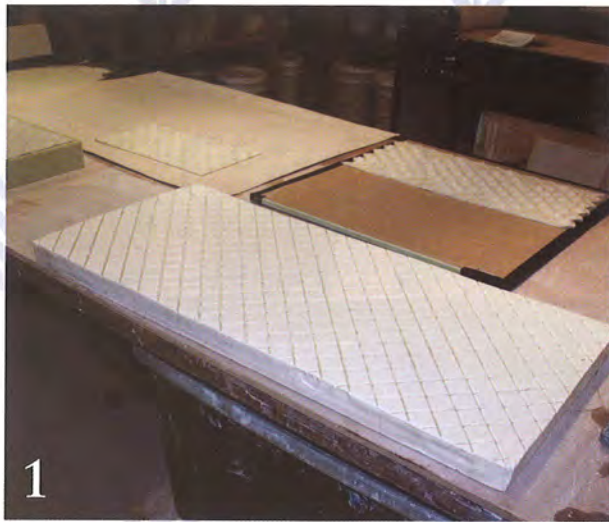
1 The double tiered vase uses two cut slabs pressed from a carved plaster block.
