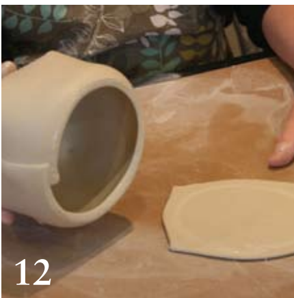
12 Make a print with slip on the slab for the bottom of the pot.
